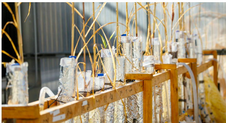
Column experiments are utilized to study nitrate transport and biogeochemical transformation in the vadose zone.
