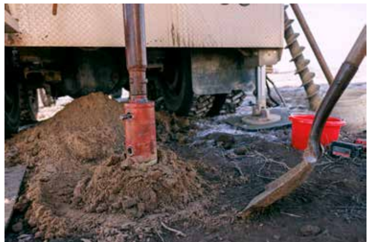
Vadose zone coring uses columns of soil samples to better understand how contaminants move underground over time.
