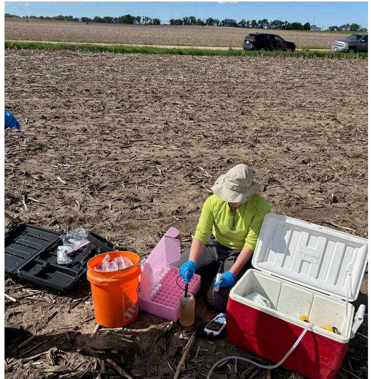
UNL graduate student Kalley Collins measuring dissolved oxygen (DO) in lysimeter water samples from field experiment where olivine was applied.
