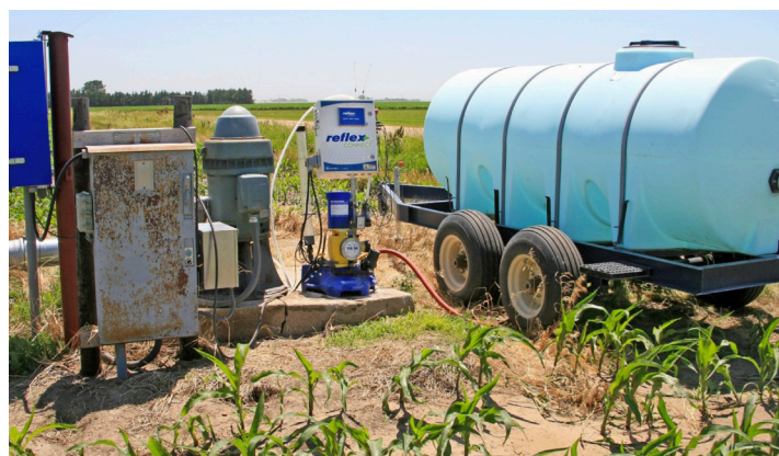
A fertigation system with programmable injection pump, used for in-season nitrogen management.
