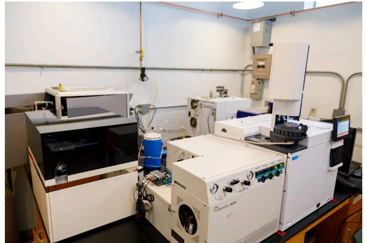
The compound specific isotope analyzer is comprised of four units that work in tandem to test water, soil, and biological tissue samples.
