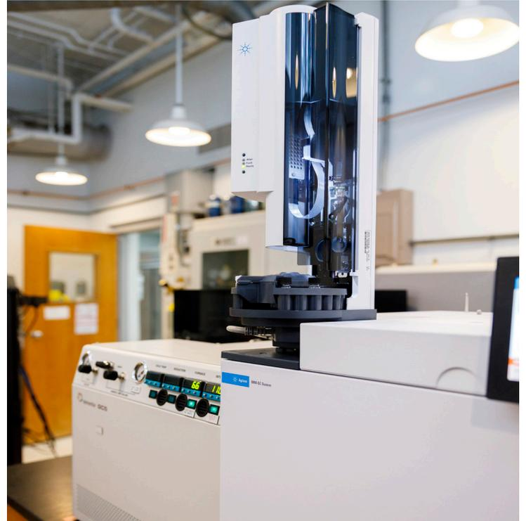
The compound specific isotope analyzer will be used for stable isotope testing.
