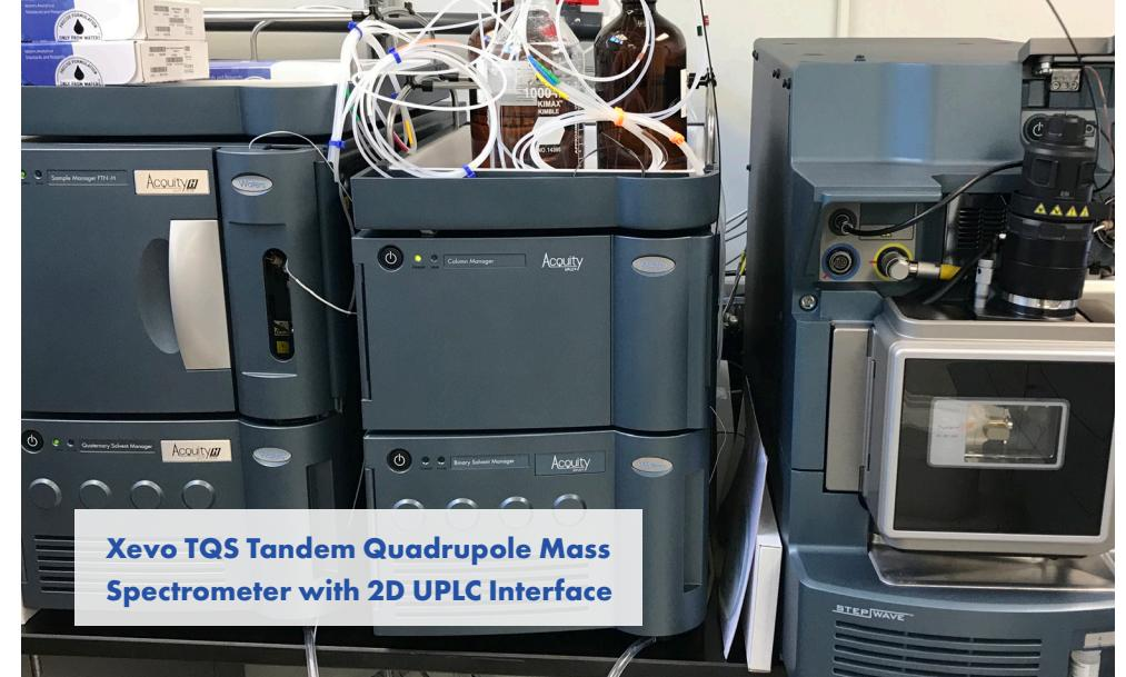
**Xevo TQS Tandem Quadrupole Mass Spectrometer with 2D UPLC Interface**
