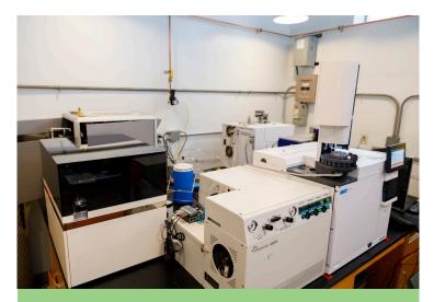
The compound specific isotope analyzer is comprised of four units that work in tandem to test water, soil, and biological tissue samples.
